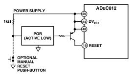
Figure 42. External Active Low POR Circuit
